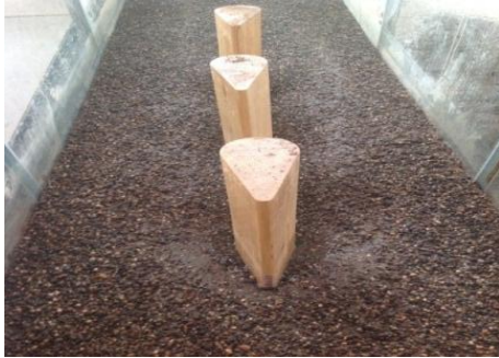
(a) Scour bed around the group of bridge piers 2-10 cm.
